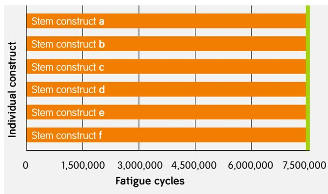
**Figure 3:** Fatigue testing results for PROMOS° STANDARD stem constructs. All stem constructs (a–f) reached the maximum number of cycles (7.5 million, shown by green line) without failure.
